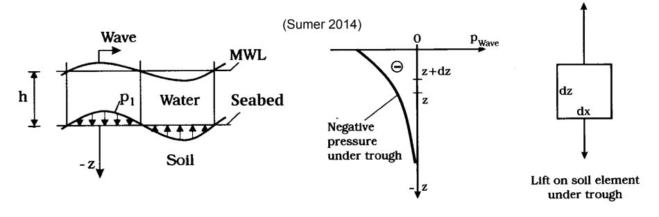
Criteria for wave-induced liquefaction of sand:  $-\frac{\partial p_{\text{wave}}}{\partial z} > (\rho_{\text{wet.sand}} - \rho_{\text{water}}) g$
