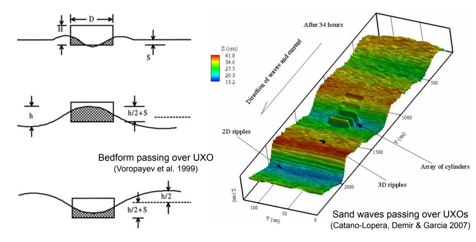
• Burial of object by bedform crest; additional object scour occurs in bedform trough.
