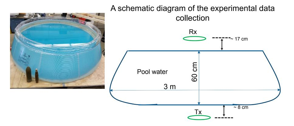
HFEMI Tx & Rx coils are about 27 cm in diameter, 12 turns. Approx distances from the coil centers to the upper and lower water surfaces are indicated.
