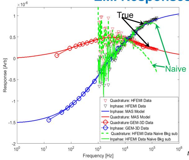
Here, a "naïve" calculation of a rocket's response simply subtracts the salt water background signal from the data, as .
