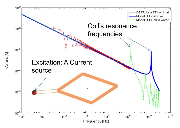
Rect: TEMTADS (TT) Tx coil: 16 Turns; total wire length 42.5 m; Excitation: A Current source
