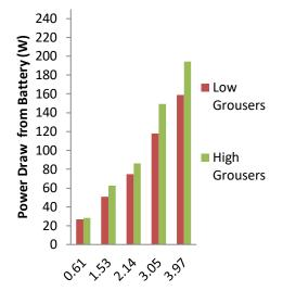
Vehicle Speed (mph) Based on Encoder Count
