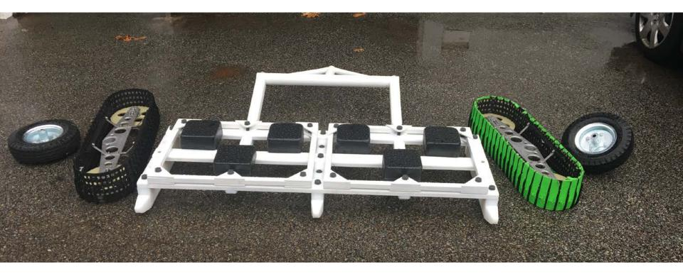
Tested various sled systems: Tweel Wheel Tracked Skid Castor
