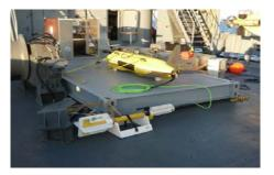
**AUV with R2Sonic & BOSS** Sonar >SeaHorse (SOAM) >Survey in waters >5 meters
