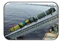
LSG/REMUS 600 > Laser Scalar Gradiometer (LSG) > EdgeTech Sidescan > Electro-Optic (EO) Imager > EdgeTech Sub-bottom Profiler
