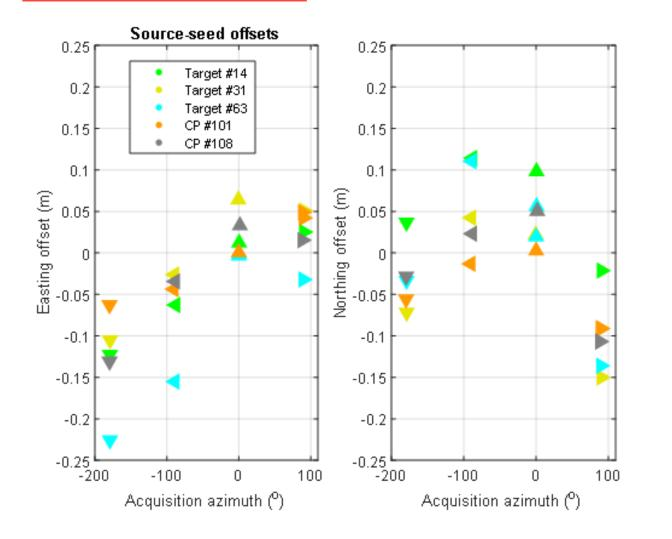
Here cued data were collected in the 4 cardinal directions over 5 targets scattered over a property. The data were subsequently inverted to predict the buried target location.
