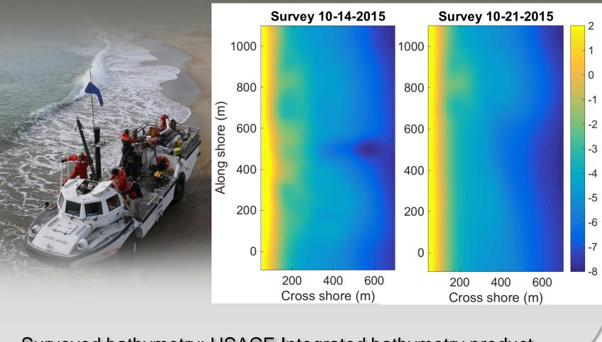
Surveyed bathymetry: USACE Integrated bathymetry product
