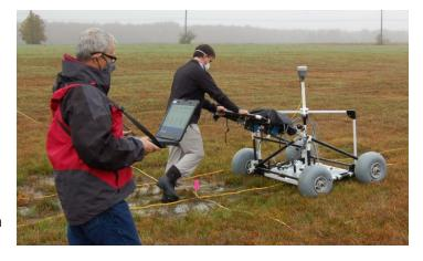
Jacobs has been working to apply Simultaneous Localization and Mapping (SLAM) positioning technology for use with the MetalMapper 2x2 advanced geophysical classification (AGC) sensor. The intent is for high quality and high accuracy location, detection, and classification of Munitions and Explosives of Concern (MEC) in GPS-denied areas, where application of AGC is limited to few and less-efficient positioning systems. Results to date from a 5ac pilot study indicate that
