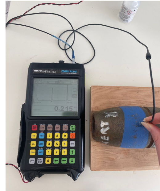
NDT: Olympus Panametrics-NDT 25MX PLUS Transducer: Olympus M116, 20/0.125"
