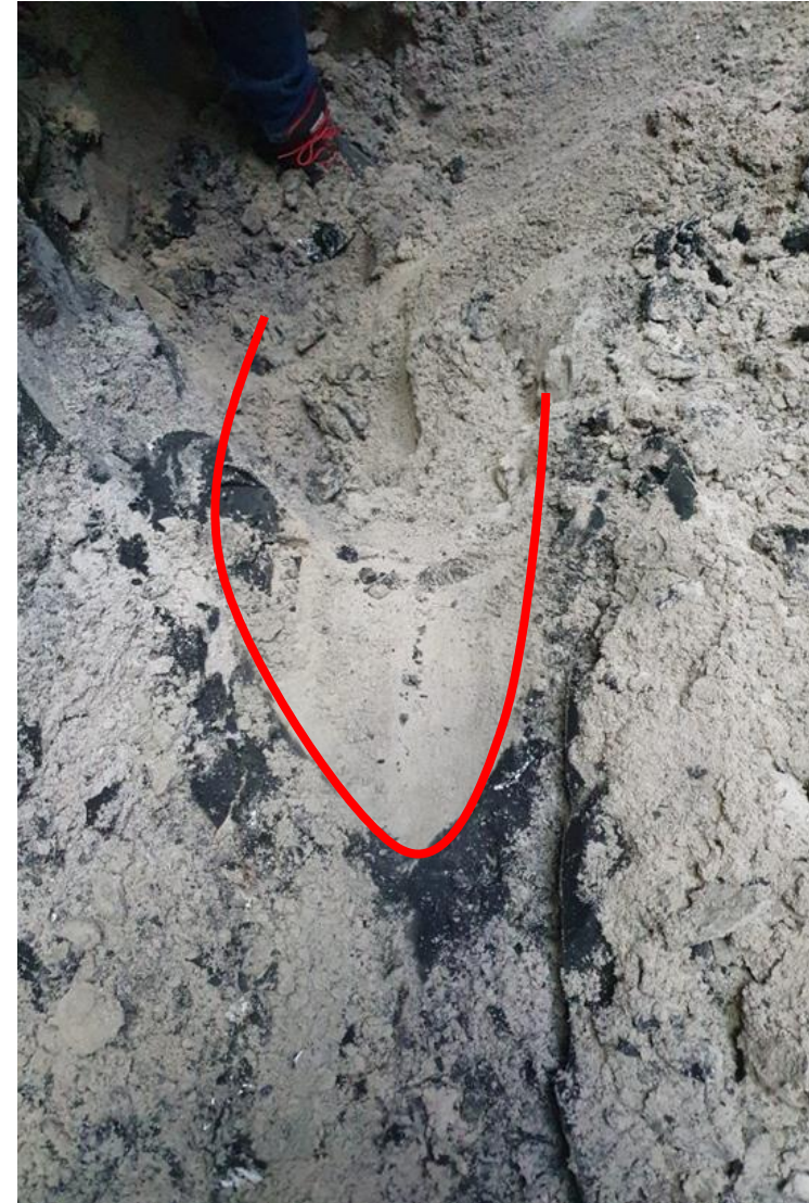
Proof of offset: approx. 50 cm above the actual unexploded ordnance find – clear marking of the bomb in the overlying layer of earth
